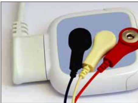
Example of a wearable waterproof ambulatory ECG medical monitoring device with three leads
